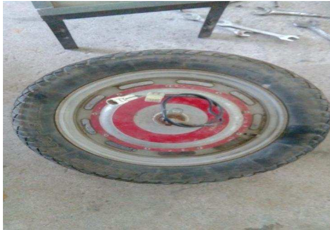
Figure 2: Hub motor (Brushless DC Motor)
